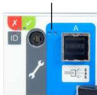
Figure 2-9 I/O module SAS Activity LED location
