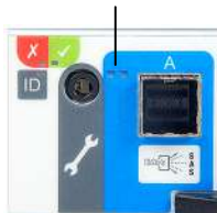
Figure 2-9 I/O module SAS Activity LED location
